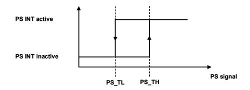
10 PS\_TH & PS\_TL (PS high & low threshold) are active as outside detection:
