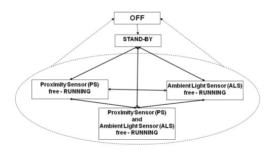
If VDD exceeds the threshold voltage, the sensor will switch from OFF mode to STAND-BY mode. As shown in the transitiondiagram above it is possible to switch between all modes without any restriction.
