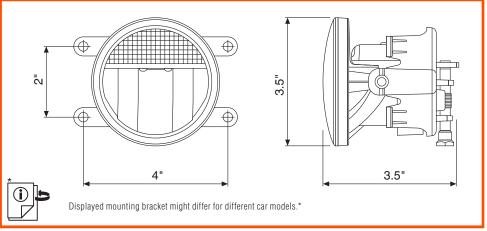
Not suitable for vehicles with standard turn indicators integrated in the fog-lamp.
