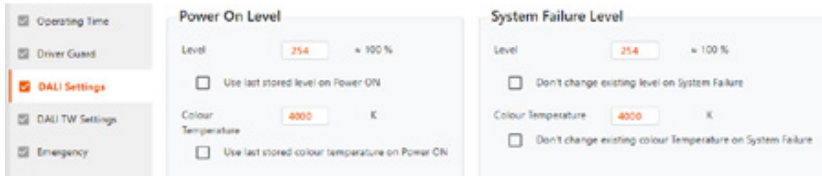
Tuner4TRONIC®: Input of initial operating conditions
