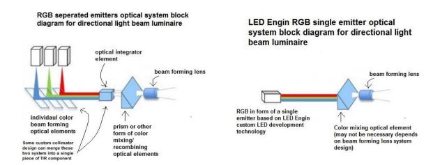
Figure 2: Simplicity of optical design when co-locating LEDs of different wavelengths in a single package
