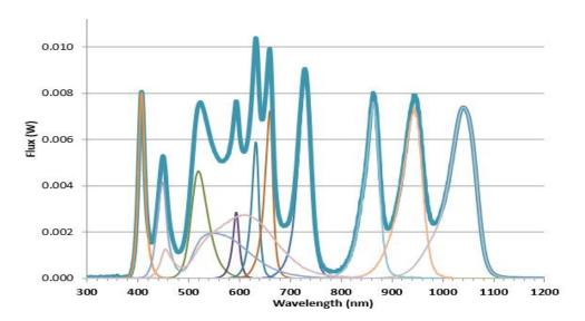
Figure 3: Spectral power distribution of an exemplary multispectral emitter
