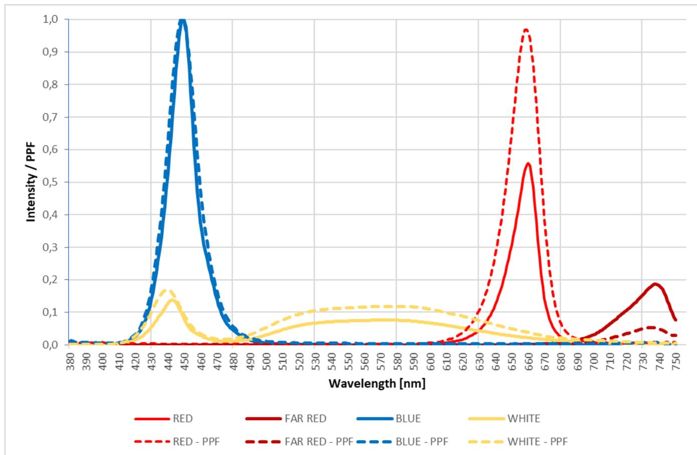
Normalized spectrum graph of the red, far red, blue and white LEDs at 350 mA current. Spectrum can be changed by choosing LEDs and power output.
