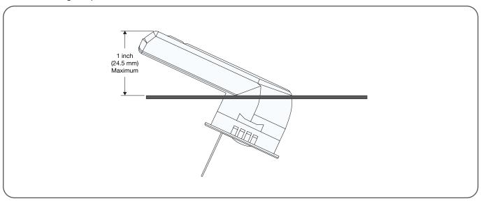
Minimum Requirements for Placing the Pre-Drilled Hole
