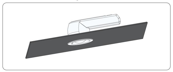
3 Push the clip towards the sensor until curved metal piece is clamped into the sensor groove.
