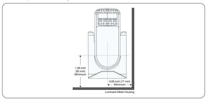
1 Push the sensor through the pre-drilled 0.5 inch (Pg-7) trade size (0.875 inch ±0.01 inch or 22.25 mm ±0.25 mm) hole.
