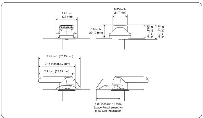
2 Minimum height required in luminaires to mount the sensor.
