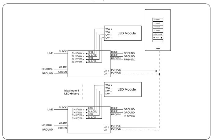
When connecting to the wallstation, control wires should be inserted into the left two push-in connectors on the back of the wallstation. Power to the wallstation and communication to and from the wallstation is achieved using these two wires only. The two ports on the right are non-functioning terminals.
