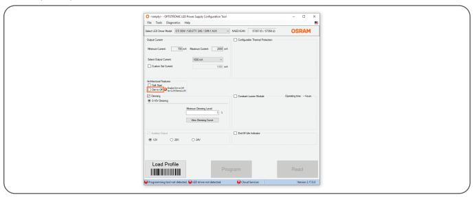
Important: When using the SensiLUM with a 0-10V LED driver, the LED driver must posses Dim-to-OFF capability, and it must be enabled.
