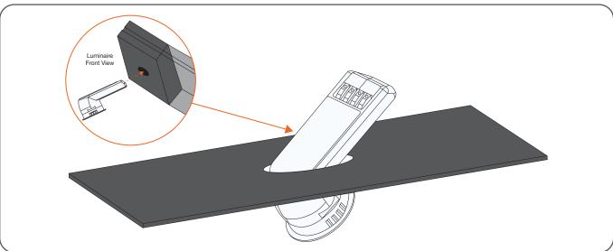
2 Position the sensor flush to the luminaire metal casing.
