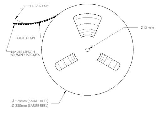
Figure 13: Emitter reel specifications (mm).
