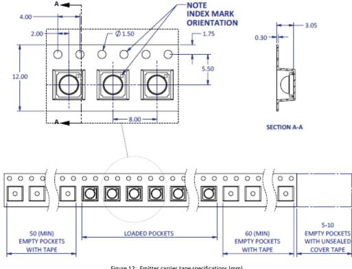
Figure 12: Emitter carrier tape specifications (mm).
