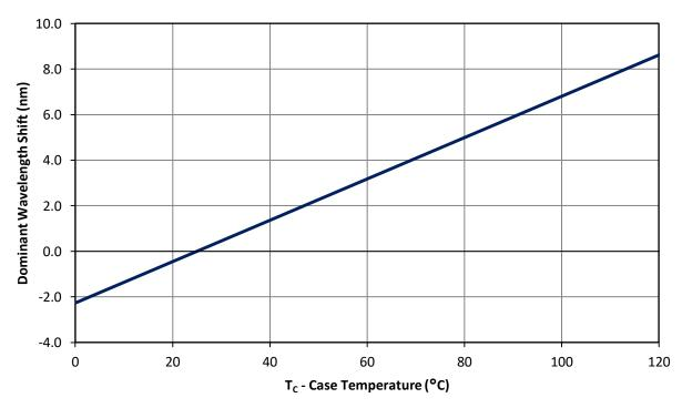
Figure 10: Typical relative dominant wavelength shift vs. case temperature.
