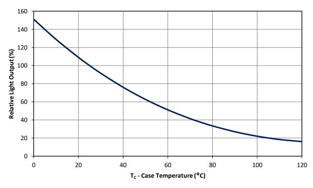
Figure 8: Typical relative light output vs. case temperature.
