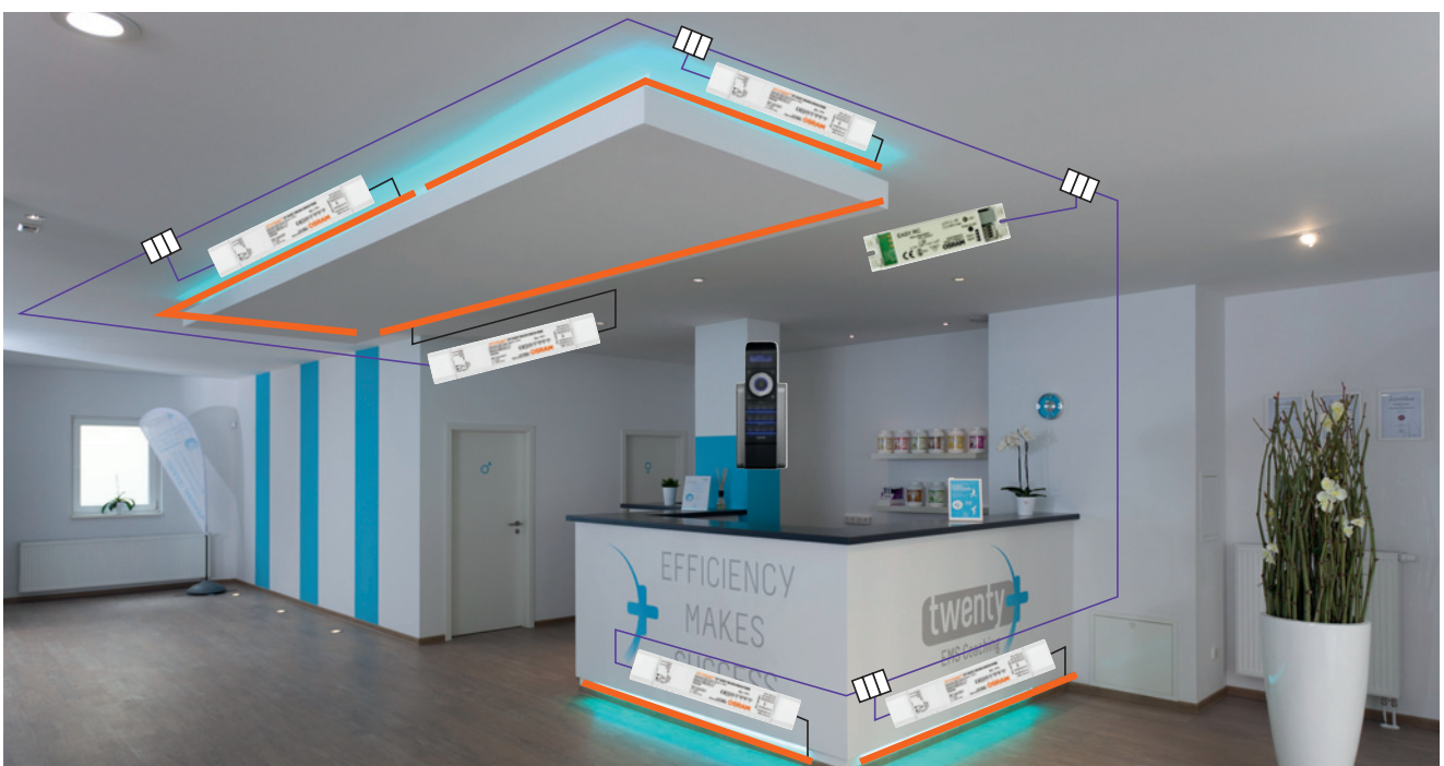
Reception area with control components
