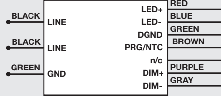
Wiring diagram 85W (347-480) w/o AUX
